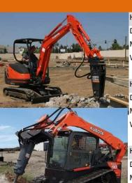
Hydraulic Breaker, 400#, Excavator Mount
